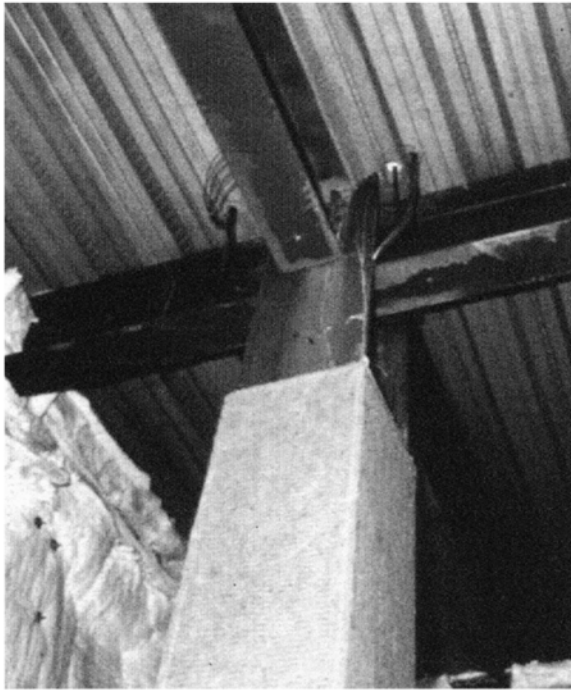
Figure 3.30 Fire protection of columns in Corus plane frame test (Courtesy of B.R.Kirby, Corus Fire Engineering).
